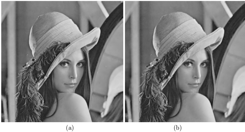
Figure 7: The test image compressed (a) by a factor of 56.60 with 40.37dB PSNR and \delta = 32 , \Delta = 64 , \varepsilon = 2.4 , d_{max} = 3 (b) by a factor of 141 with 45.74dB PSNR and \delta = 64 , \Delta = 128 , \varepsilon = 2.6 , d_{max} = 3 using the bivariate model.
